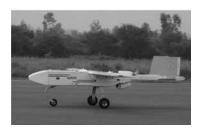
operators as the turnaround time between sorties can be significantly reduced. The Panchi has all the surveillance capabilities of the Nishant, but it can stay in the air longer because it does not have to carry the airbag and parachute systems of the Nishant. It is also a light vehicle with its body made of composites, and has a high degree of stealth because it has a low radar cross-section signature. Having an endurance of four hours, it can track ground targets over an area of 165 km.
