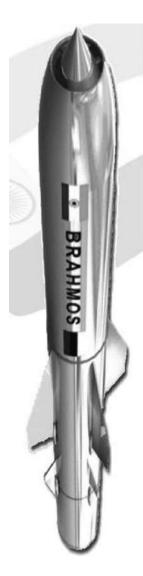
BRAHMOS is a two-stage missile with a solid propellant booster engine as its first stage which brings it to supersonic speed and then gets separated. The liquid ramjet or the second stage then takes the missile closer to 3 Mach speed in cruise phase. Stealth technology and guidance system with advanced embedded software provides the missile with special features.
