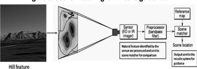
Figure 8. Scene matching for missile guidance.36
