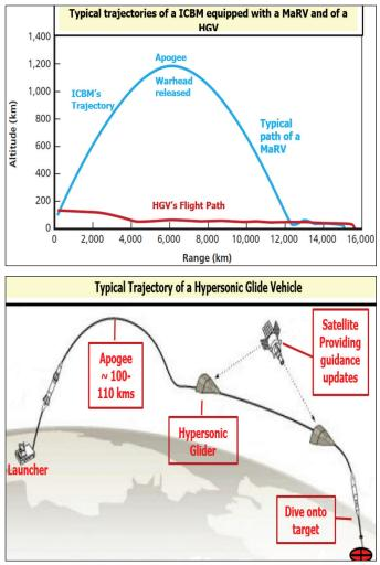
or some form of terminal guidance is provided. HGVs, on the other hand, do not rise above 100–110 km altitude and spend over 80–100 percent of their flight time below 100 km altitude (i.e. within the atmosphere).
