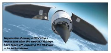
trajectory to the target. Thereafter, the HGV starts to fall back to Earth, gaining more speed and gliding along the upper atmosphere, before diving on the target.
